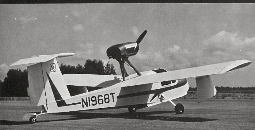
Engine mount is cantilever truss, rear is open for quick access. You can walk on hull top to get to powerplant and propeller.
